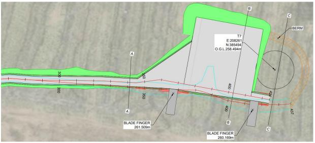
Figure 147 T7 Turbine and Hardstanding plan
