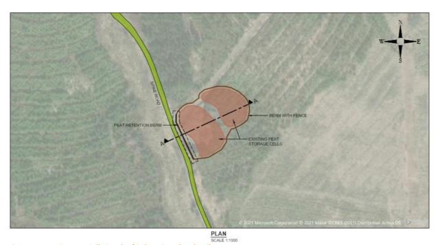
Figure 17 Peat Storage Cells South of Substation plan details
